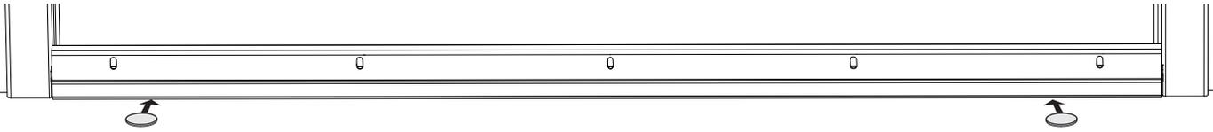
6. **AFFIX SWEEP TO DOOR USING MOUNTING SCREWS(B)** WITH EITHER #2 PHILLIPS OR HEX BIT. PLACE SCREWS NEAR TOPS OF SLOTS ON SWEEP. **TIP: ONLY FULLY TIGHTEN 2 OUTERMOST SCREWS.**
