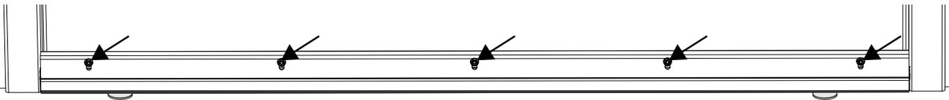
7. **CHECK DOOR SWING** AFTER REMOVING SHIMS BY OPENING AND CLOSING THE DOOR SEVERAL TIMES, TAKE NOTE OF ANY EXCESSIVE DRAGGING OR WEDGING. IF NEEDED LOOSEN SCREW ON PROBLEMATIC SIDE, SLIGHTLY LIFT SWEEP, AND RETIGHTEN. REPEAT UNTIL DOOR SWINGS FREELY. **NOTE: FOR MAXIMUM EFFECTIVENESS AGAINST PESTS & THE ELEMENTS GAP SHOULD BE AS NARROW AS POSSIBLE.**
