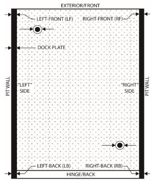
Measure gap from LEVELER TOE GUARDS or TOP PLATE to PIT WALL, excluding retainers or shims. THESE SHOULD BE REMOVED DURING INSTALL!
